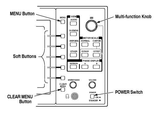
Figure 8: Controls for initial power up and configuration
